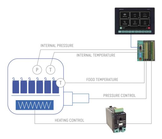
The main characteristics of these applications are the archiving of process values during the sterilization cycle and the calculation of F0, i.e., the time equivalent to sterilization temperature. F0 calculation lets you automatically check, ensure, and certify the quality parameters of the treated product.
