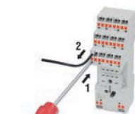
Cable removal with screwdriver
