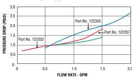
Tests conducted with units in vertical position (lead wires up) with water
