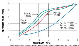
Tests conducted with units in a horizontal position with water at +70°F (21°C). Data will vary slightly for vertically mounted units.
