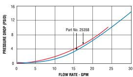
Tests conducted with units in horizontal position with water at +70°F (21°C). Data will vary slightly for vertically mounted units.
