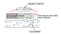
An externally rotatable vane is positioned in the main flow path within the unit. The magnet carrier piston is located in a bypass flow chamber. Pressure differential, caused by flow around the adjusting vane, displaces the spring-biased piston which actuates a hermetically sealed SPDT reed switch within the unit.
